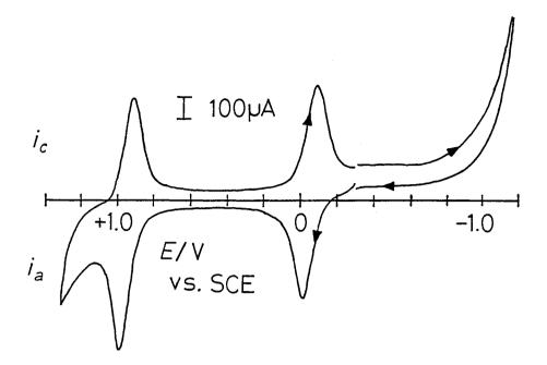
Fig. 1. Cyclic voltammetric response of  $[Ru^{III}_3(\mu_3-O)(\mu-CH_3COO)_6(pyridine)_2(CH_3OH)]^+$  incorporated poly(4-vinylpyridine) film on a glassy carbon electrode, in aqueous Na(CF<sub>3</sub>COO) medium(0.1 M, pH 3) with an SCE and a Pt wire. Scan rate: 20 mV s<sup>-1</sup>.
